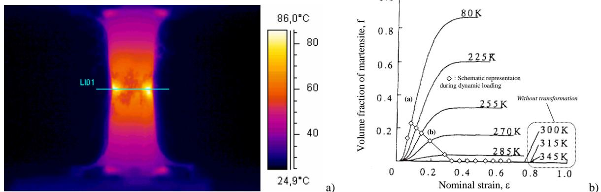
Fig.3. a – Temperature measurement during quasi-static tensile loading,  $\dot{\epsilon} = 10^{-2} \text{ s}^{-1}$  and  $t = 27.4 \text{ s}$ , b - Kinetics of phase transformation versus strain for different initial temperatures [2]
