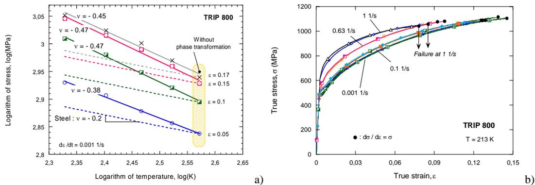
Fig.2. a – Temperature sensitivity in quasi-static loading, b – Strain rate sensitivity at low temperature,  $T = 213 \text{ K}$
