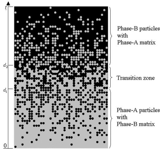
Fig. 1 Schematic illustration of a two-phase FGM sample
