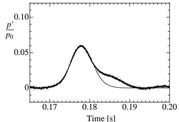
**Figure 2.** Temporal pressure profiles at a position distant about 5.2 m from the piston where the thick and thin lines indicate the profile measured and the one of the solitary wave, respectively.
