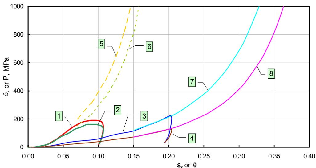
Fig. 5. Examples of "stress  $\sigma$  - strain  $\epsilon_x$ " curves for wet (1 & 2) and dry (3 & 4) sand obtained from SHPB tests, and "pressure  $P_i$  - volumetric strain  $\theta$ " curves for wet (5 & 6) and dry (7 & 8) sand from plane-shock wave tests
