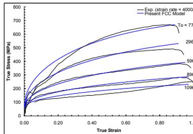
Figure 2 Adiabatic stress-strain curves, for the proposed fcc model, for OFHC Copper, and compared to the experimental results at  $4000 \text{ s}^{-1}$  strain rate and for different initial temperatures.
