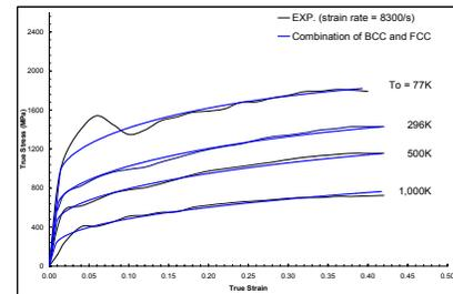
Figure 3 Adiabatic stress-strain curves, for the proposed models, for AL-6XN stainless steel, compared to the experimental results at  $8300 \text{ s}^{-1}$  strain rate and for different initial temperatures.
