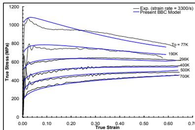
Figure 1 Adiabatic stress-strain curves for the proposed bcc model, for Niobium (Nb), and compared to the experimental results at  $3300 \text{ s}^{-1}$  strain rate and for different initial temperatures.
