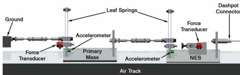
Figure 1. Experimental fixture for nonlinear energy pumping.
