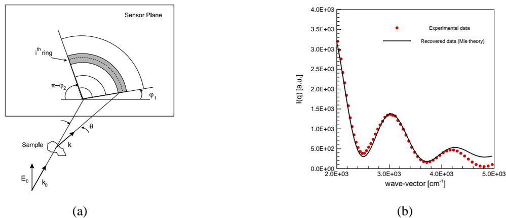
**Figure 2.** (a) Schematic representation of a typical detector for LAELS measurements; (b) Comparison between experimental and reconstructed angular intensity distributions in the case of iso-propanol droplets with an average diameter of  $54 \mu\text{m}$ .
