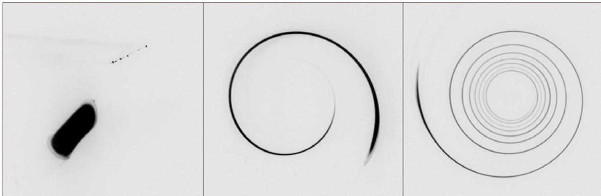
**Fig. 1:** Roll-up of a blob of fluorescent dye in a point vortex at  $t = 0, 2$  and  $10$  s. The field of view is  $4.8$  cm wide.
