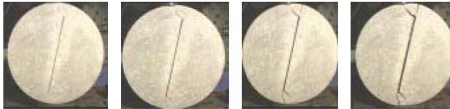
Fig.6 crack propagation trajectory of Brazilian disk specimens
