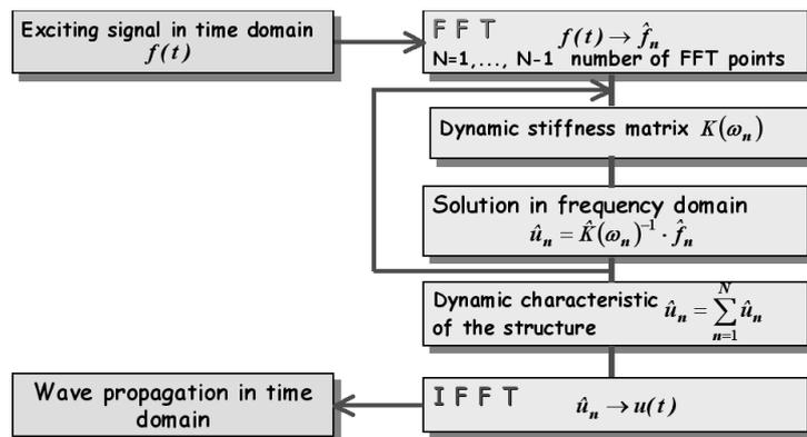
Figure 2. Flow diagram for the wave reconstruction program.
