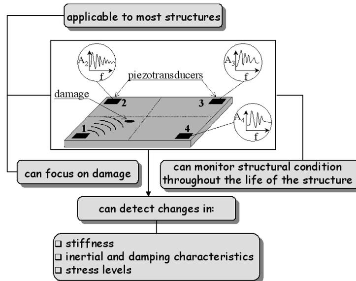
Figure 1. Build in sensor network on a plate.
