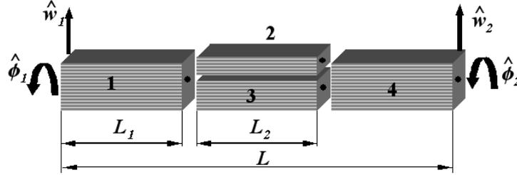
Figure 5. Model of a composite beam with delamination.
