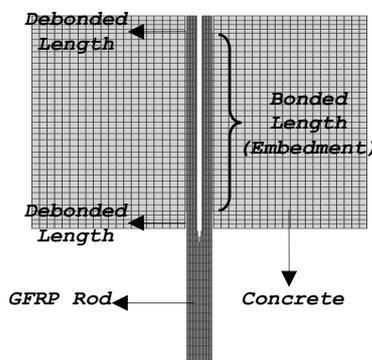
Figure 1- Typical shape of the axisymmetric FE model.
