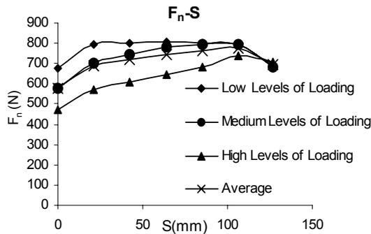
Figure 4- Variation of  $F_n$  along the embedment.
