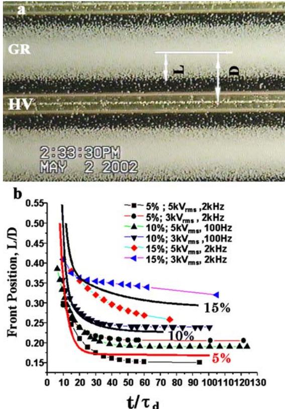
**Figure 2.** (a) The photo illustrates how the front location was measured; HV and GR refer to the high-voltage and grounded electrode respectively. (b) The experimental data (symbols) and computational results (solid lines) for the front propagation in 5, 10, and 15% (v/v) suspensions [8].
