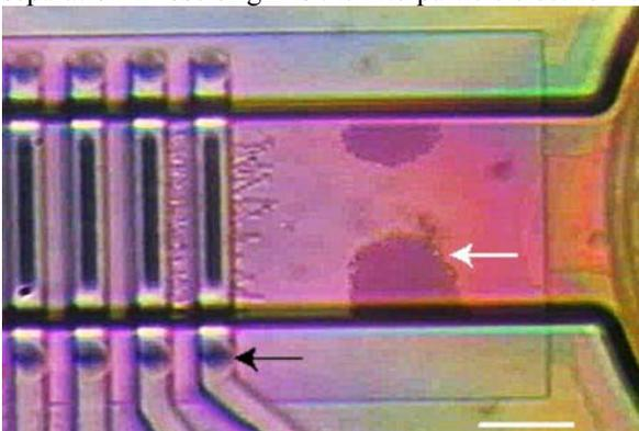
**Figure 1.** Dielectrophoretic (10V<sub>ptp</sub>, 15MHz) separation of bacterial cells and beads. The cells adhere to the energized electrode (black arrow) while the beads experience negative dielectrophoresis accompanied by a phase separation (white arrow). The flow is from right to left. Scale bar = 20  $\mu\text{m}$  [6].
