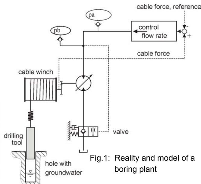
The first step for solving these problems consisted in considering the hydraulic and mechanical model of Fig. 1 and in deriving the corresponding equations of motion [1,2]. For this we must take into account the hydraulic and the mechanical degrees of freedom together with the appropriate bilateral and unilateral constraints as given by the configuration itself as well as by hydraulic or mechanical non-smooth features. We
