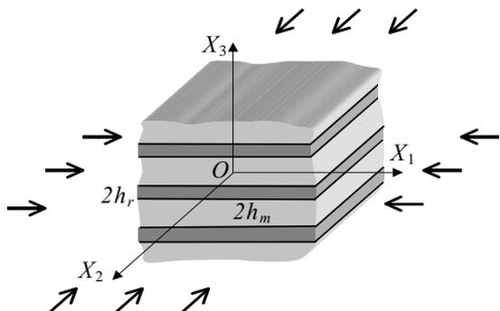
Fig. 1: The co-ordinate system and applied loads.
