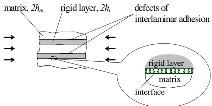
Fig. 2: An interface with a cleavage-type delamination.
