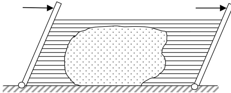
**Fig.** A plane scheme of the device. The figure plane is parallel to the plane of shearing and to the planes of two smooth side walls (not represented), the latter closing side openings of the cavity
