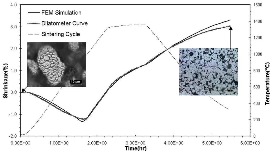
**Figure 1.** Comparison of the FEM simulation and dilatometry plots on axial shrinkage versus temperature for a stainless steel 316L presintered compact heated at a rate of 10 C/min to 1350 C in hydrogen (powder mean size 52.5µm).
