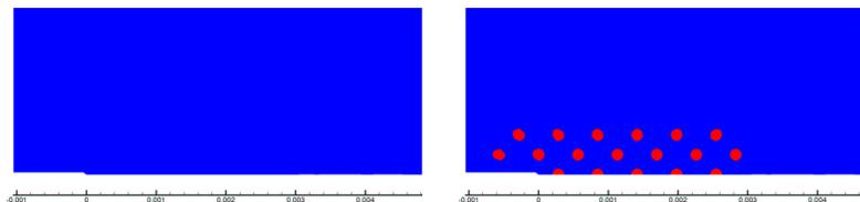
**Figure 1.** Contours of the amplitude of stress-controlled void nucleation in the near crack tip region showing the inclusion distribution for two slices of  $y^3 = \text{constant}$ .
