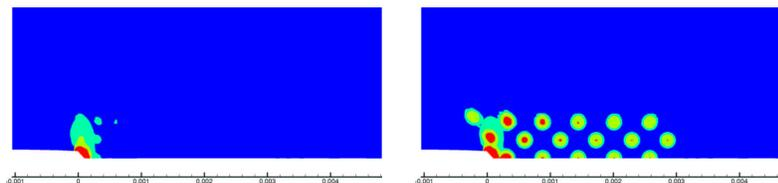
**Figure 2.** Contours of void volume fraction in the near crack tip region for the two slices of  $y^3 = \text{constant}$  in Fig. 1.
