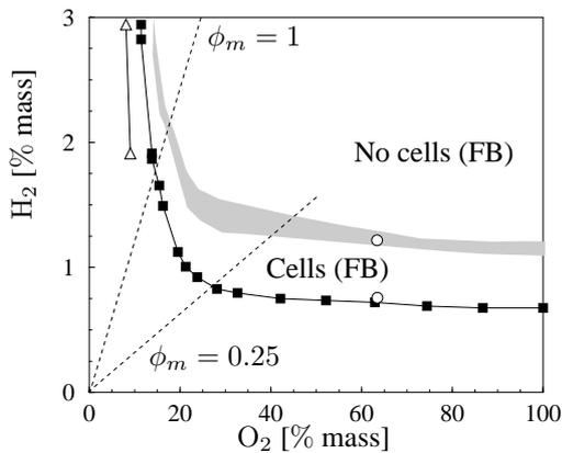
**Figure 2.** Near-extinction limits and region of cellular instability in nearly unstrained planar non-premixed CO<sub>2</sub>-diluted H<sub>2</sub>-O<sub>2</sub> flames; Shaded region: transition from non-cellular to cellular flames for the FB configuration; —■—: FB near-extinction limit; —△—: FT near-extinction limit; ○: conditions for Fig. 3.
