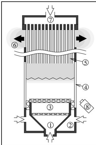
**Figure 1.** Schematic of the burner. (1) bottom reactant flow, (2) inert co-flow, (3) porous plates, (4) fused silica windows, (5) tube array for reactant supply from top, (6) hot product exhaust, (7) top reactant flow, (8) movie camera.
