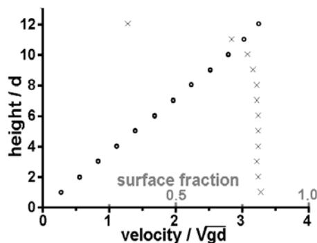
**Figure 2.** Corresponding adimensioned velocity profile and solid fraction (averaged over 100 samplings).
