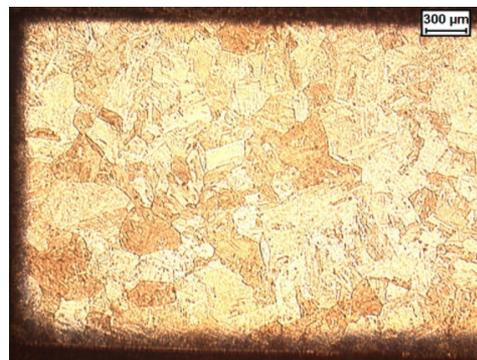
**Figure 4.** Austenitic grain of steel A after 10h at 1000°C ( $\approx$  200-300  $\mu$ m in diameter)
