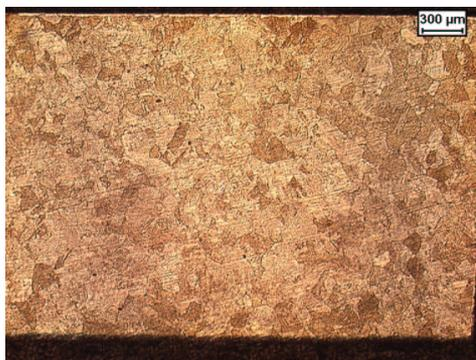
**Figure 3.** Austenitic grain of steel A after 10h at 1000°C ( $\approx$  100-150  $\mu$ m in diameter)
