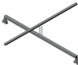
Fig. 2 Beam-on-beam collision with a local contact spring
