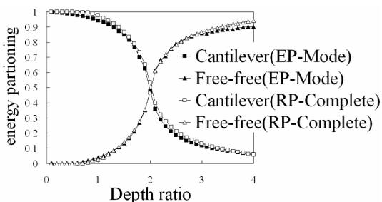
Fig. 1 Energy partitioning between two beams
