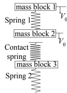
Fig. 3 A simple mass-spring collision system
