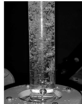
Fig. 2. Vibrational injection of gas into fluid
