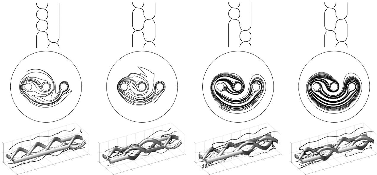
**Figure 1.** Example results of dye advection in the BSD (middle row) and BPM (bottom row), with stirring regimes corresponding to different braid topologies (top row). In the BSD the flow topology refers to how the stirring rods are moved around each other; in the BPM the topology describes how the internal pipes are intertwined. The images show the fate of a straight line initial dye blob after a ‘moderate’ stirring time.
