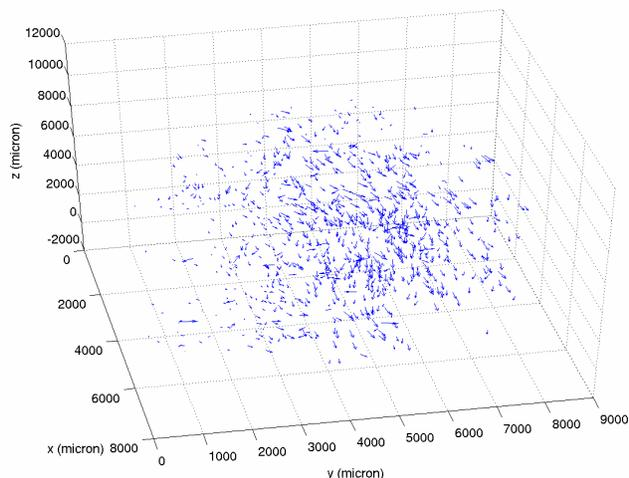
**Figure 5:** Extracted HPIV vectors from figure 4, the jet is flowing from top to bottom.
