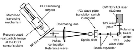
**Figure 3:** Reconstruction of two sequentially multiplexed polarization holograms using circular polarization wave.
