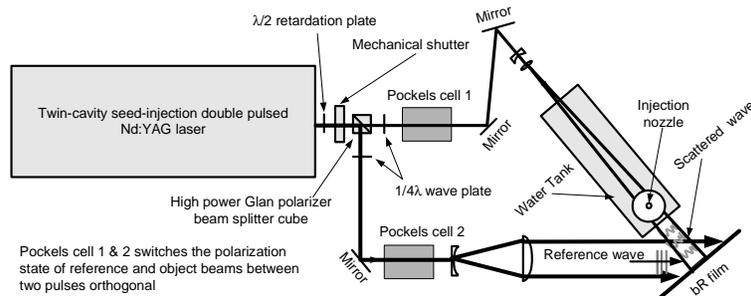
**Figure 2:** Schematic of the recording setup for the HPIV experiment.
