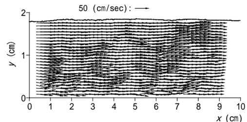
Figure 1 Instantaneous velocity vectors with the corresponding water surface profile ( $Re_* = 505$ ,  $Fr = 1.23$ ).
