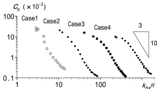
Figure 4 Streamwise spectrum of the water surface fluctuation. The values in horizontal axis are modified by multiplying 5, 5<sup>2</sup>, 5<sup>3</sup> in Case2, 3, 4, respectively.  $Fr = 0.54, 0.64, 0.85, 1.23$  in Case1,2,3,4, respectively.
