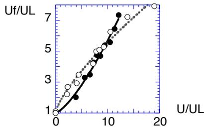
**Figure 2.** Relative increase of front velocity  $U_f/U_L$  as a function of the relative flow intensity  $U/U_L$  in convective flows (full circles) and in electroconvective flows (open circles).
