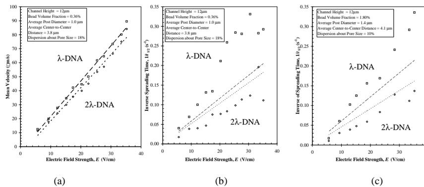
Figure 2: Comparison of theory and experiment for the mean velocity (a) and band broadening (b,c) for the matrix geometries indicated in the insets. Short dashed lines (theory) and  $\square$  (experiment) refer to  $\lambda$  DNA; long dashed lines (theory) and  $\diamond$  (experiment) refer to  $2\lambda$  DNA.
