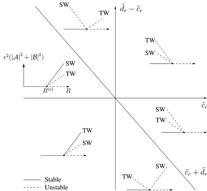
Figure 1. Bifurcation diagrams in the  $(\tilde{c}_r, \tilde{d}_r - \tilde{c}_r)$  plane, showing the amplitude  $\epsilon^2(|\mathcal{A}|^2 + |\mathcal{B}|^2)$  of travelling waves (TW) and standing waves (SW) as a function of the Rayleigh number  $R$ . Here,  $\tilde{c}_r = (c/a)_r$ ,  $\tilde{d}_r = (d/a)_r$ , and the subscript  $r$  indicates the real part.
