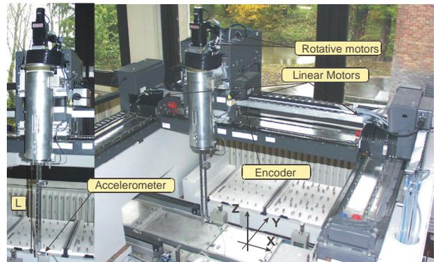
Fig. 1: Set-up: pick-and-place machine.
