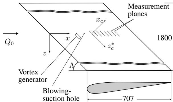
Figure 1. The swept wing model. Dimensions are in mm.
