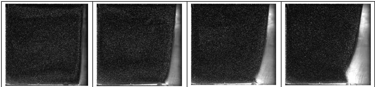
Fig.2. Experimental pictures: the seed and the temporal solid-liquid front position after 100s, 500s, 1000s and 2000s (from left to right) of solidification of 3.5%wt aqueous solution of NH<sub>4</sub>Cl.
