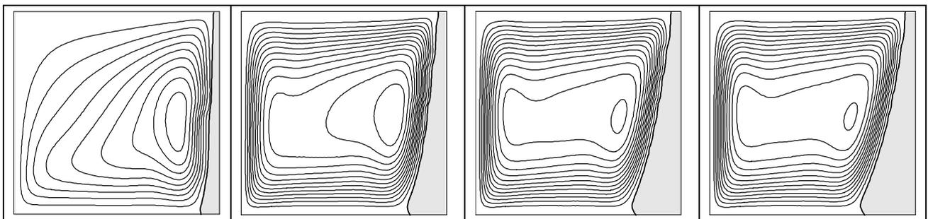
Fig.3 Enthalpy-porous medium model: the calculated flow pattern and solid phase shape after 100s, 500s, 1000s and 2000s (from left to right) of solidification of 3.5%wt aqueous solution of NH<sub>4</sub>Cl.
