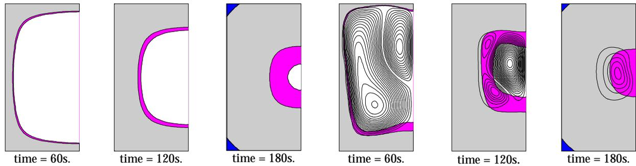
Fig.1. Solidification of Al<sub>2</sub>wt%Cu in a sand mould: white – liquid phase, pink – under-cooled liquid zone, grey – mushy zone, dark blue- solid phase.
