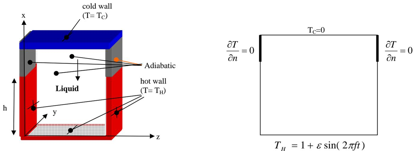
**Figure. 1** : Geometrical configuration - 3D full domain and 2D domain.
