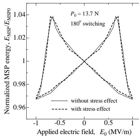
Fig.3 MSP energy vs electric field for applied force
