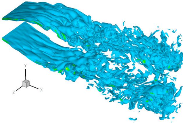
**Figure 2.** Instantaneous vorticity isosurfaces of LES of a plane underexpanded jet.
