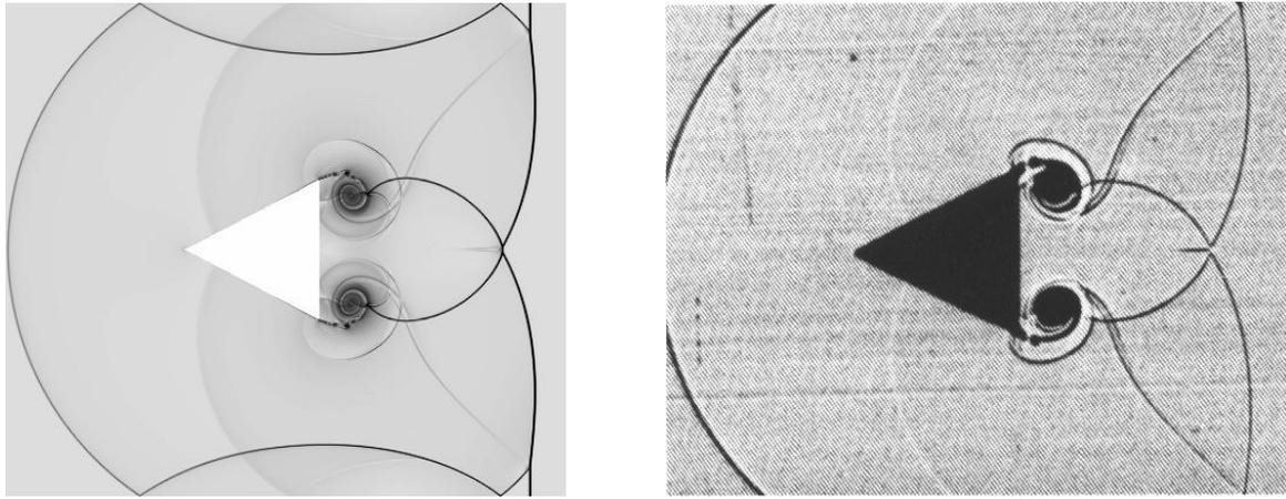
**Figure 1.** Numerical schlieren picture (left) and experimental shadowgraph (right) of shock wave diffraction on a finite wedge.
