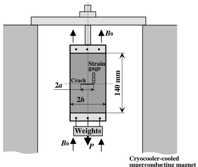
Fig. 2 Testing set-up
