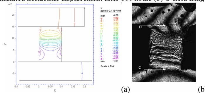
Figure 3 (a) Simulated vertical displacement after 600 hours (b) V field fringe after 605 hours
