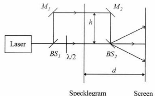
Fig.2. Schematic of the optical pointwise filtering method
