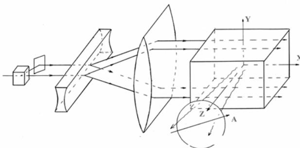
Fig.1. Schematic of optical slicing method.
