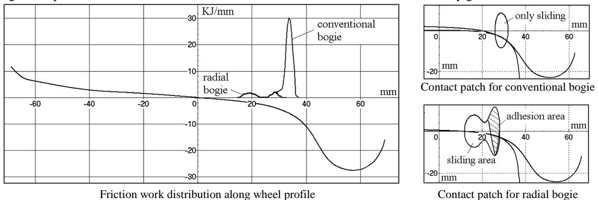
Figure 3. Results of railway simulation in even curve.
