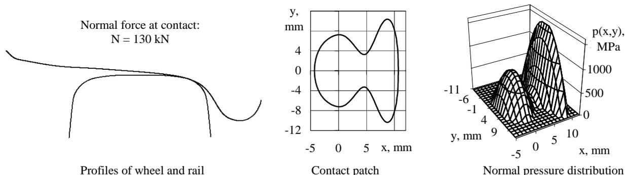
Figure 1. Example of normal contact problem solution.
