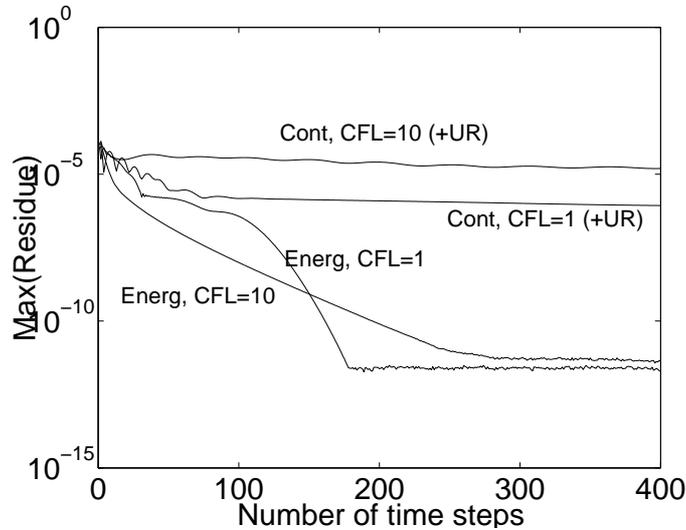
**Figure 1.** Subsonic nozzle flow,  $M_{throat} = 0.001$ . Convergence plot for computations at convective CFL numbers of 1 and 10. *Energ*: Mach-uniform algorithm. *Cont*: equivalent algorithm based on the continuity equation (computation with underrelaxation (UR))
