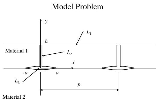
Figure 1. Initiation and growth of Interface cracks.
