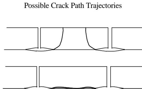
Figure 2. Illustration of possible crack path trajectories
