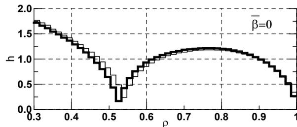
Figure 4. Distribution of dimensionless thickness  $h(\rho)$  of annular plate with immovably clumped inner edge, movably simply supported and loaded outer edge.
