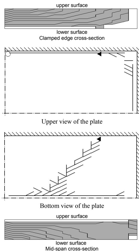
**Figure 1:** Cracking patterns at time  $t_2$ .
