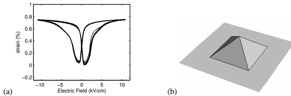
**Figure 1.** (a) Large electrostriction in BaTiO<sub>3</sub>. (b) A tent-like actuated shape of a large displacement actuator.
