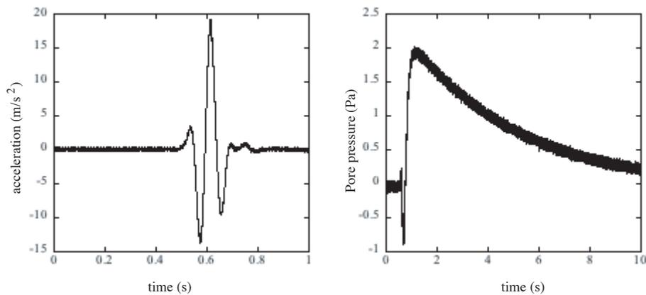
**Figure 2.** Acceleration (left) and pore pressure relaxation (right) versus time for a 2 cm high packing of 112  $\mu\text{m}$  glass spheres.
