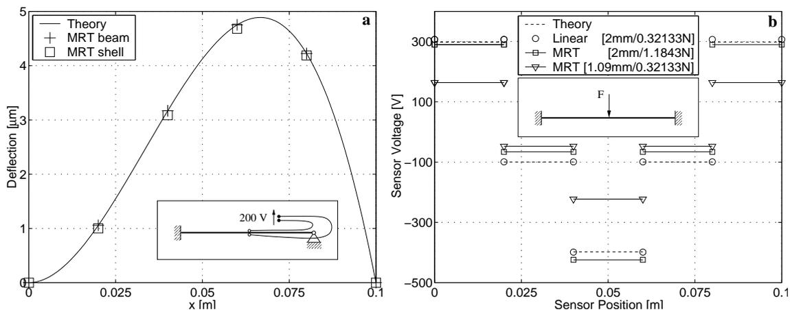
**Figure 1.** a: bimorph beam acting as an actuator with 200V. b: bimorph beam acting as sensor with a mid-point displacement of 2mm.
