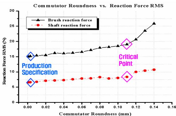
Fig. 2 Graph of Commutator roundness vs. Reaction force
