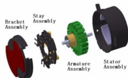
Fig. 1 3D CAD Model of DC motor
