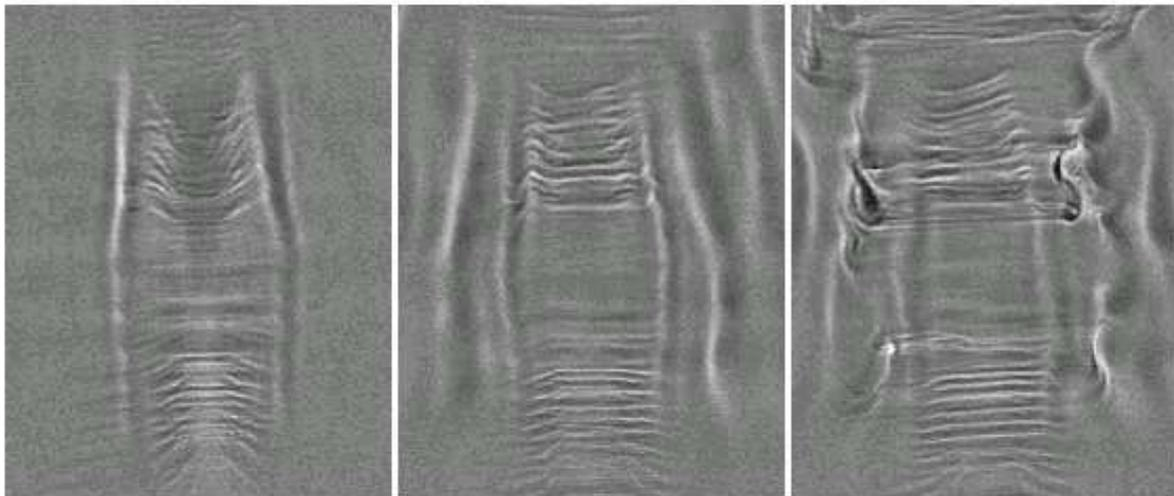
**Figure 1.** Shadowgraph pictures of inertia gravity waves, emitted by an oscillating cylinder at the right side of the vortex near the bottom, breaking in the shear flow of a tall vortex. The cylinder diameter is  $D = 5.0$  cm, while oscillation frequency and amplitude are  $0.88s^{-1}$  and  $1.0$  cm respectively, and  $N_0/f = 1.5$ . Times of observation are: 79, 123 and 137 s after forcing.
