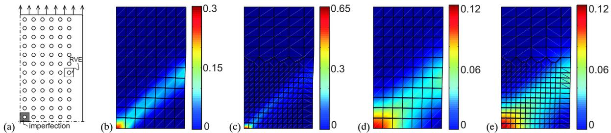
**Figure 1.** Homogenization analysis of a macroscopic localization problem. Geometry (a) and the strain distribution obtained by the first-order (b), (c) and second-order (d), (e) computational homogenization analysis using two finite element discretizations.
