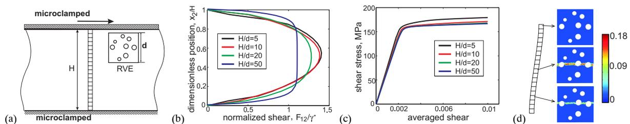
**Figure 2.** Homogenization analysis of the macroscopic boundary shear layer problem. Geometry (a), distribution of shear across the height of the macroscopic strip (b), shear stress-strain response (c) and microstructural deformation patterns in the sheared macroscopic layer for  $H/d = 5$  (displacements are 10 times magnified).
