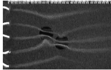
Fig.2. Interaction of two fixed circular cavities of an equal radius  $R_0 = 18$  mm, center-to-center distance  $l = 2.5R_0$ , and angle of attack  $30^\circ$ . Granular material is glass beads of a diameter 1mm. Flow visualization by sodium fluorescein.
