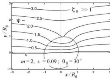
Fig.1. Streamlines around a slightly deformed cylindrical cavity:  $r = R_0[1 + \epsilon \cos[m(\theta - \theta_0)]]$ ,  $m = 2, \epsilon = 0.09$ , angle of attack  $\theta_0 = 30^\circ$ ,  $\zeta_0 \gg 1$ .
