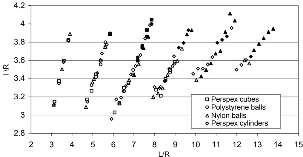
**FIG. 2** A compendium of all data gathered in the investigation of the dependence of periodic length ( $l$ ) on tube length ( $L$ ) for particles suspended in water (full markers represent observed oscillations between two possible band patterns). The coordinates are scaled by tube radius in-order to manifest general features of the banding phenomenon.
